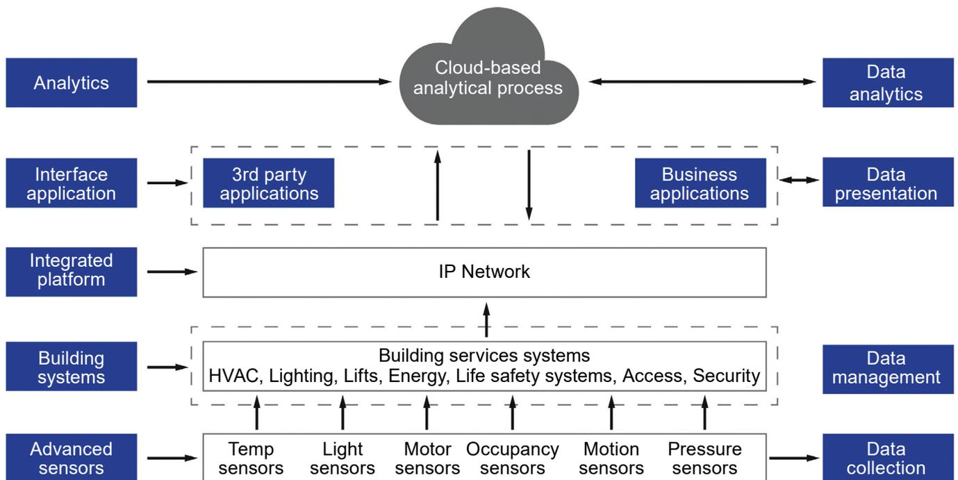
**FIGURE 4:** IoT intelligent connected building.
