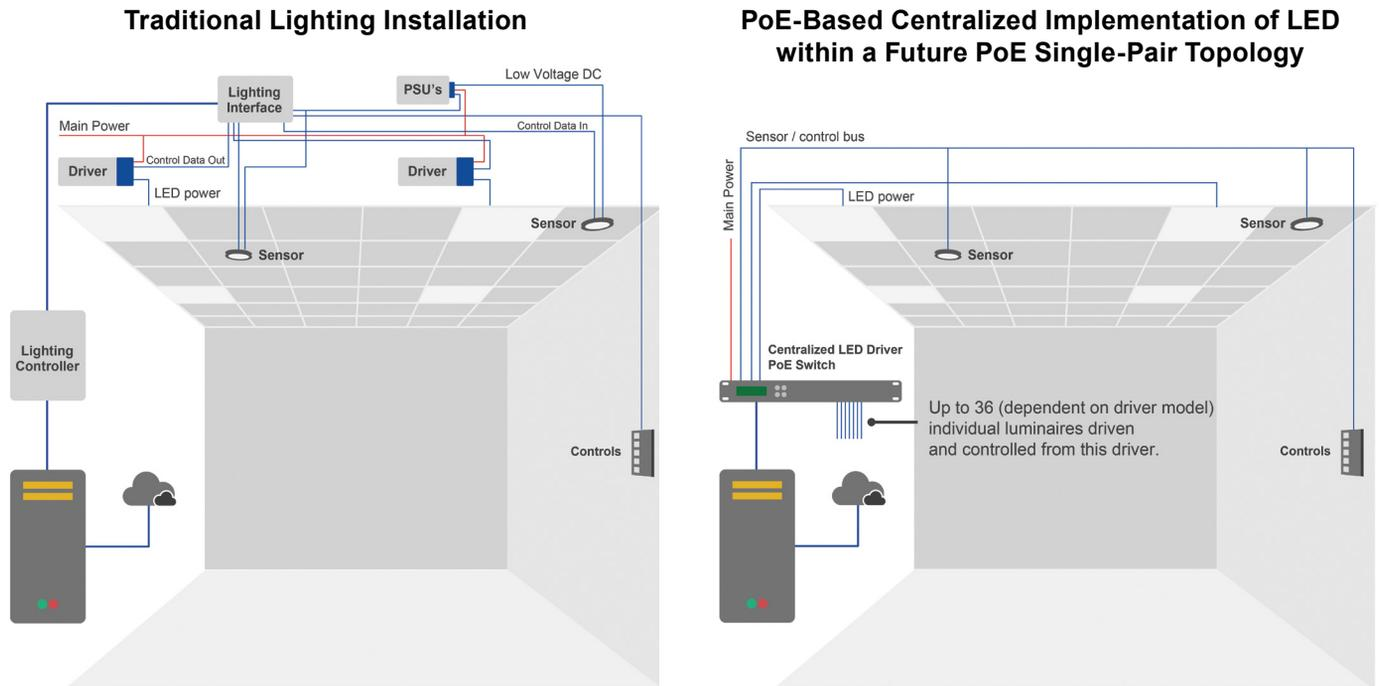
**FIGURE 2:** Classic LED lighting versus PoE-based lighting within a future PoE single-pair implementation.
