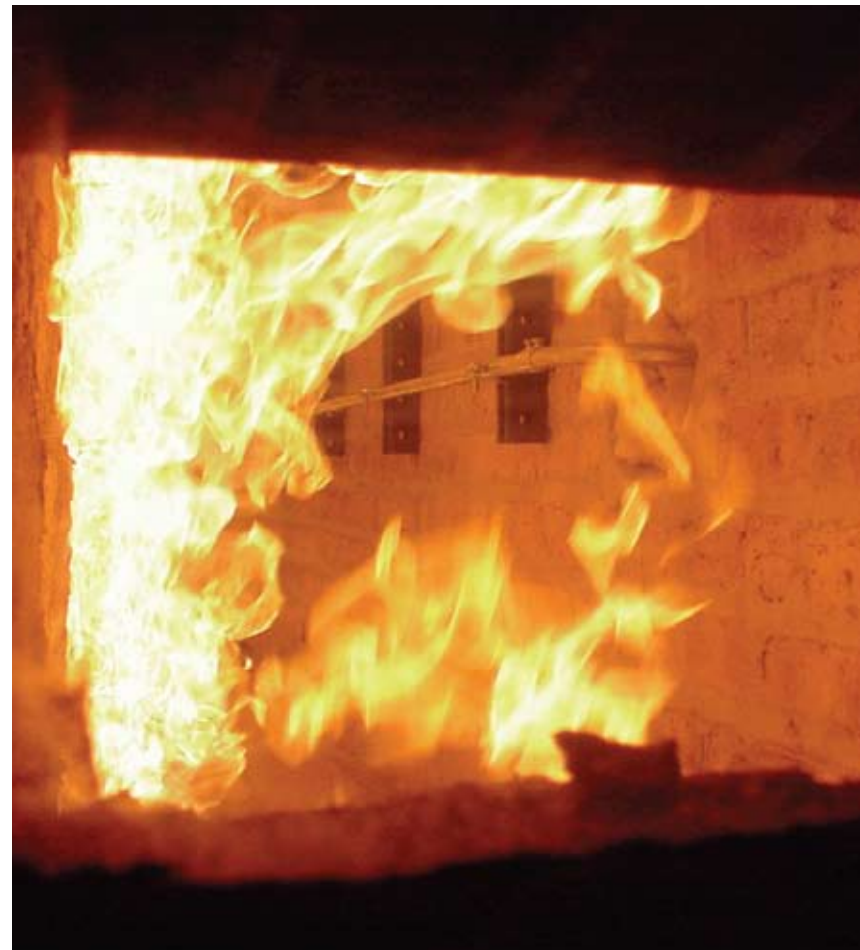
Lifeline cable undergoing UL 2196 testing
