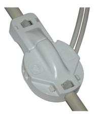
The Verticasa Mini Branching Unit is typically used in multi dwelling units to breakout and distribute the fibres from an in-line Verticasa cable into a drop tube, for routing to a customer premise. It has the capacity to accommodate Verticasa cables of up to 9mm in diameter. It enables a window to be cut in the cable to access the fibres, which can be spurred of into drop tubes of 3mm in diameter (8 positions) or a drop tube of 5mm in diameter (2 positions).
