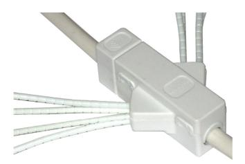
The Verticasa Breakout Unit – 8 Port is typically used in multi dwelling units to breakout and distribute the fibres from an in-line Verticasa cable into a drop tube, for routing to a customer premise. It has the capacity to accommodate Verticasa cables of up to 12mm in diameter. It enables a window to be cut in the cable to access the fibres, which can be spurred of into a drop tube of 3mm in diameter.
