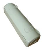
The Verticasa Cable Protection Cover is typically used in multi dwelling units or office fibre cabling systems. It is used to cover and protect the window cut in a Verticasa cable. The unit can accommodate Verticasa cables of up to 15mm in diameter.
