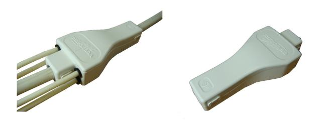
The Verticasa Breakout Unit – 4 Port is typically used in multi dwelling units to breakout and distribute the fibres from an in-line Verticasa cable into drop tubes, for routing to a customer premise. It has the capacity to accommodate Verticasa cables of up to 15mm in diameter. It enables a window to be cut in the cable to access the fibres, which can be spurred of into drop tubes of 5mm in diameter. Up to 4 drop tubes can be accommodated.
