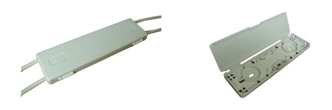
The Verticasa Mechanical Splice Holder (MSH) is mainly used for Multi Dwelling Units (MDU's) or office fibre cabling system's. The unit is suitable for splicing together up to 2 fibres (either small cables or Verticasa ESFU's). Both heat shrink and mechanical splices can be used with the MSH. Cables of up to 6mm in diameter can be accommodated.
