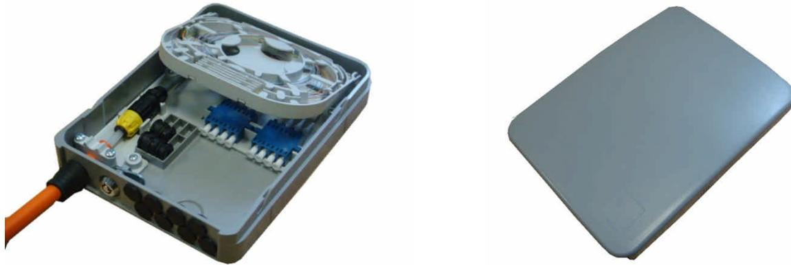
The Internal / External Compact Termination Wall Box is designed for use in residential, small and large businesses premises. The unit houses a single splice tray and allows fibres from external cables to be spliced to pigtails for connection to customer drop patch cords. The external cable enters from the bottom of the unit, with the customer drop cables (patch cords) exiting from the bottom of the unit or directly through the back of the box and through the wall.
