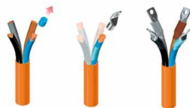
*Photo sequence shows the termination process of a Sectorflex®-type cable with the same tools used to terminate a round-shaped conductor cable.*
