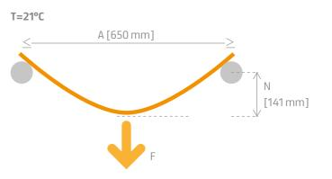
Data obtained, show a substantial improvement in the Sectorflex®-type cable handling, especially in terms of force needed to bend it, reduced by 39%. Similarly, the spring-back effect shows a reduction by more than 8%.
