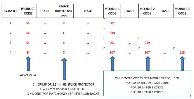
Example 1 above is for a 1U SRS Sub-Rack. The part number is **S4-H-001**. This denotes a 1U high SRS4000 Sub-Rack fitted with a blank Splice and Patch module. The sub-rack is for use with 2.2mm heat shrink splice protectors.
