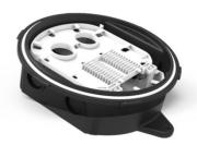
The SJC Closure is a splice closure that is used for track or branch applications. It has 4 cable entry ports, a splice cassette for 24 splices and a cable management and storage area. The closure is sealed to IP68 for water and dust tightness. The closure is supplied with four knock-out ports and two entry glands. Up to two additional entry glands can be ordered separately.
