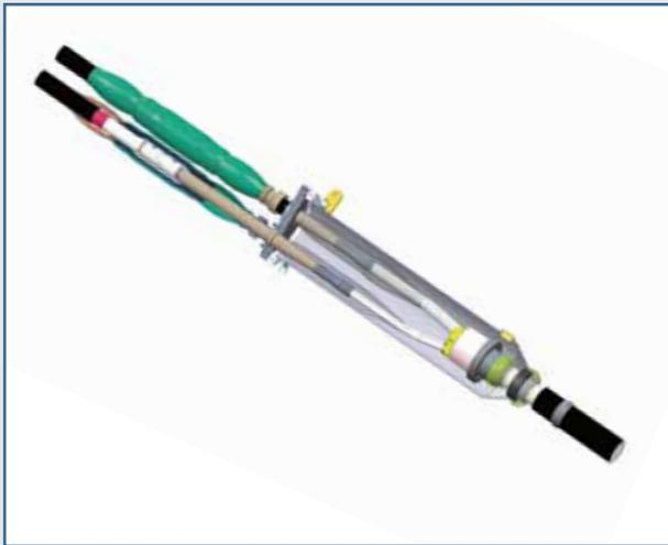
In most cable systems around the world, the 33 kV cable designs are 3 core and therefore the appropriate transition joint must be able to joint a range of 3 core fluid filled cables to 3 single cores of XLPE cables.
