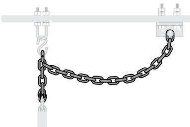
**IMPORTANT NOTE ON SAFETY AND WARRANTY FOR WHISPER-FLEX AND STEADI-FLEX:** These components are specifically designed for the installation of Whisper-Flex/Steadi-Flex cables. ONLY THE S-HOOK, MESH GRIP AND COUPLINGS ARE AVAILABLE SEPARATELY. USE OF OTHER HARDWARE (non-Draka Elevator components) COULD SERIOUSLY JEOPARDIZE THE SAFETY OF THE WHISPER-FLEX OR STEADI-FLEX CABLE INSTALLATION AND WILL VOID ANY WARRANTY.
