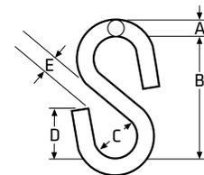
Since the S-Hook is designed to yield in order to alleviate possible damage in the event of obstruction, this item is available for replacement purposes.
