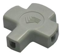
Verticasa Secondary Manifolds are used to drop fibres from a multi fibre tube to multi fibre or single fibre tubes. The secondary manifold manages the bending radius of the fibres to 15mm. There is an entry port for an input multi fibre tube of 5mm in diameter. There are drop ports for three multi fibre tubes of 5mm in diameter, and four single fibre tubes of 3mm in diameter.
