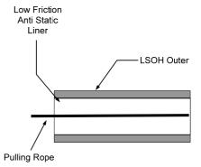
Verticasa Drop Tubes are used to route Verticasa fibre modules to the customers premises. The internal drop tube is a 5mm diameter LSOH tube with a low friction liner on the inside wall of the tube. The tube also contains a pre-installed pulling rope to make fibre installation easy.
