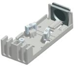
The BEM Cable Clamp is used to anchor a single cable and to distribute up to 16 cable elements (192 fibres). The BEM is suitable for cables between 36 and 192 fibres. 20 metres of routing tube is supplied with the BEM. The BEM allows for the anchoring / termination of both the cable strength member and any Aramid with in the cable construction.
